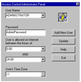
Pictured at left is the account setup dialog. When loaded it displays the Administrator's account. Users passwords may be viewed in this dialog, so it is appropriate the Administrator perform these operations while alone.
